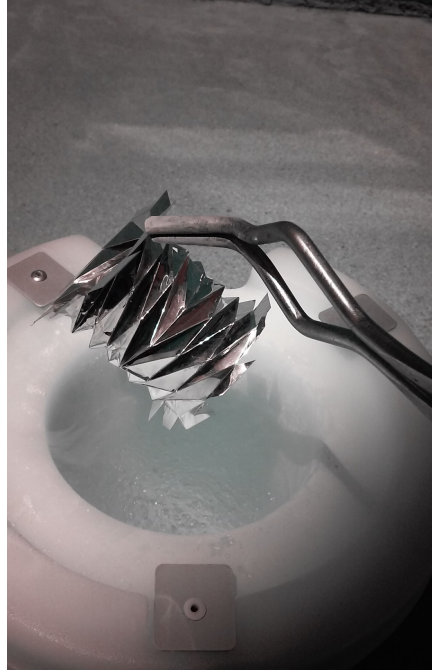
Figure 4.13: Thermal cycling the bellow's materials between liquid nitrogen and atmospheric temperatures.
