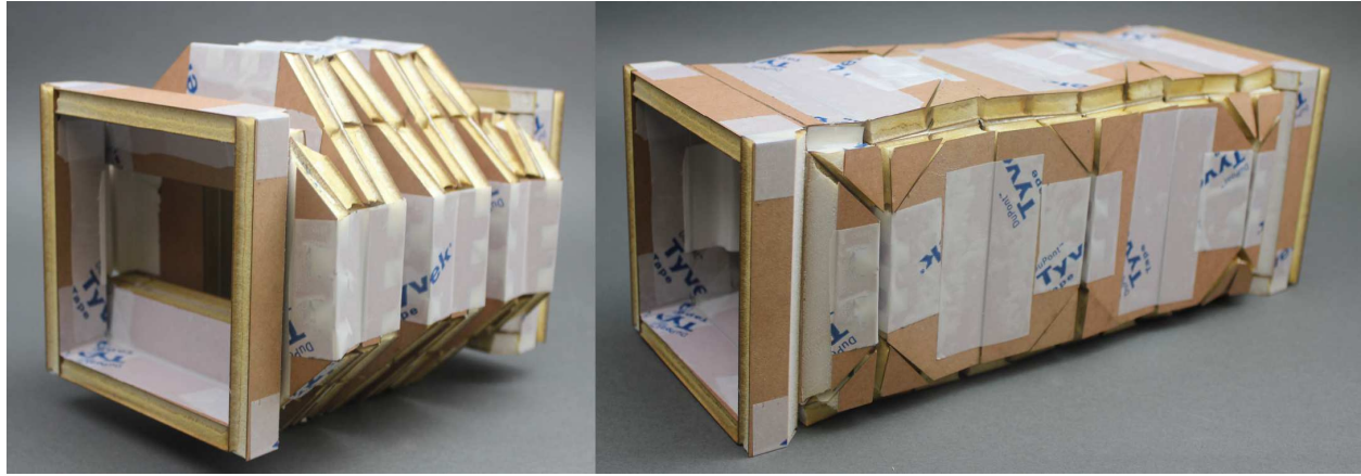
Figure 3.9: A prototype of the habitat using the modified Accordion fold pattern in thick, rigid material in both its stowed and deployed states.
