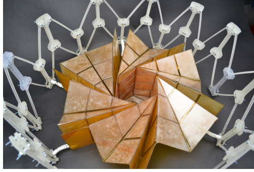
Figure 2.10: Origami-adapted solar array that modifies the crease pattern to accommodate thickness and rigid foldability.
